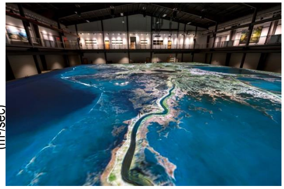
Large flume model of the Mississippi River delta at LSU
